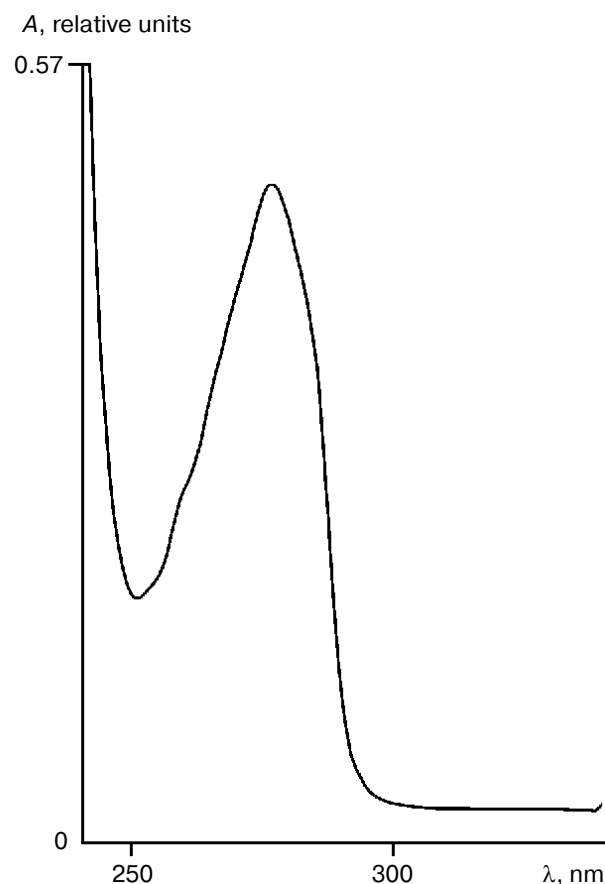
Fig. 2. Absorption spectrum of Hfq protein in the UV-range. Abscissa, the wavelengths (nm); ordinate, the absorption (optical units per 1 ml).
